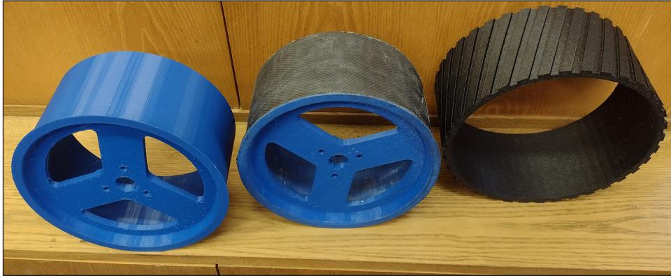
Fig. 5. PLA rim, carbon strip rim and tire
